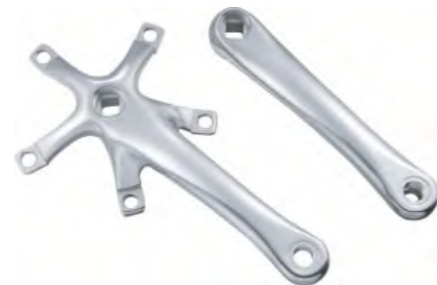
MODEL : WD130 AA LENGTH: 165-175MM BCD: 130MM
